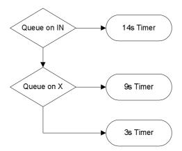
Figure 4 M271 NB Timer Selection Logic in Group Actuator
